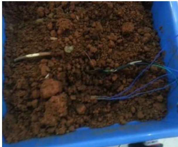
Fig.4.2: Soil with moisture and temperature sensor
