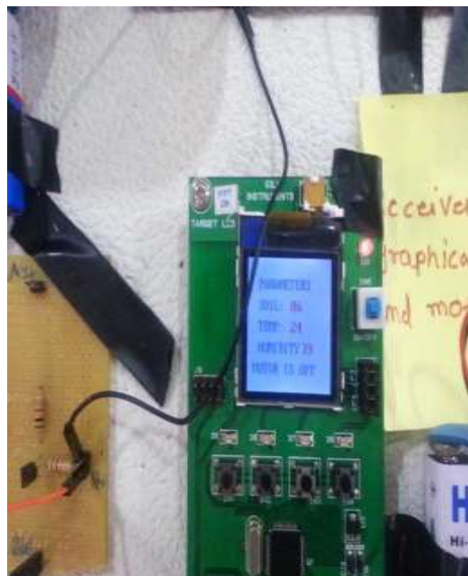
Fig. 4.4: Receiver with display showing all data
